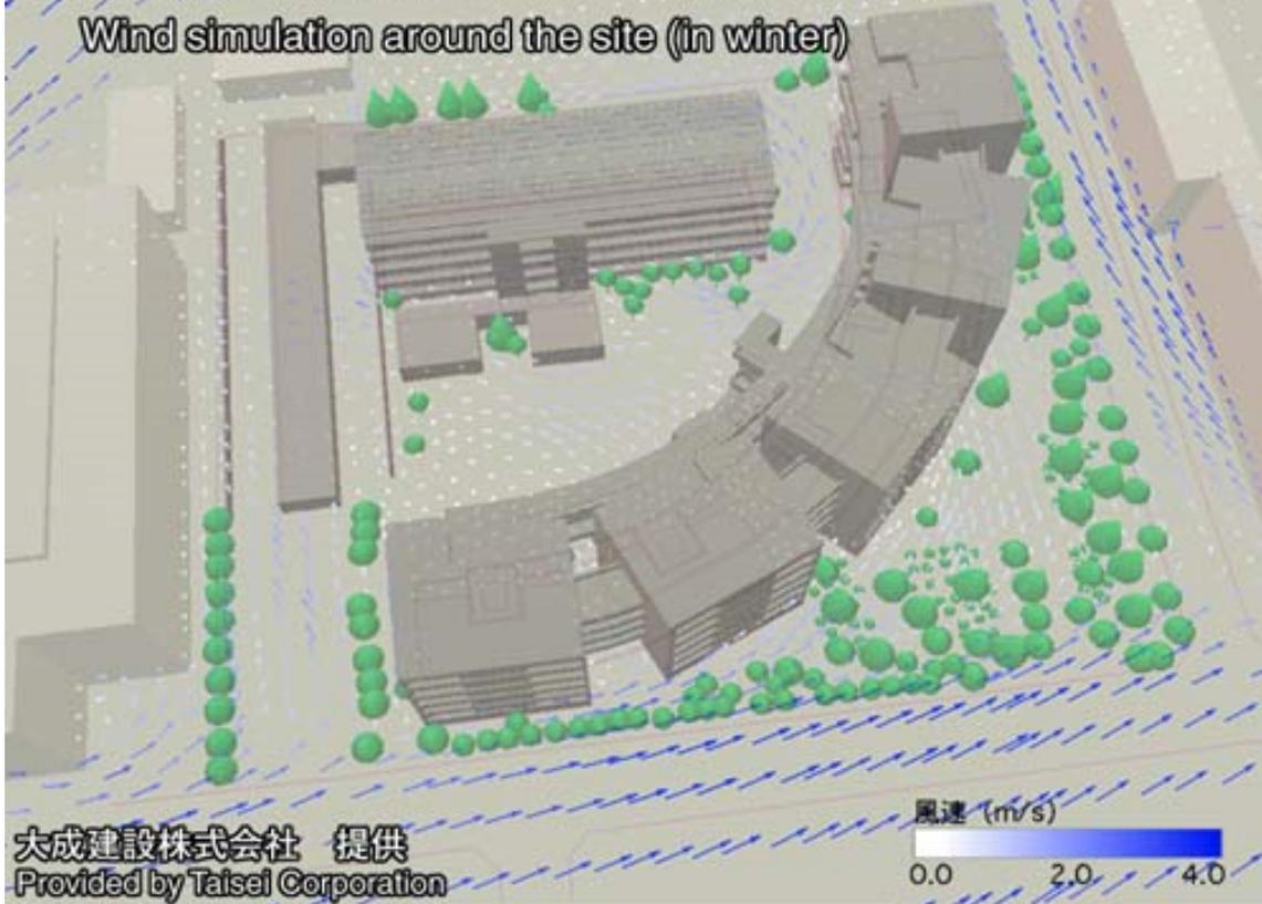
Lay out of apartments and trees, in accordance with the result of simulation, could regulate wind movements in favor of residential comfort.
